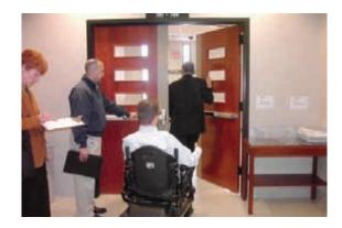
The remodeled courtrooms all have a ramp to the jury box and witness stand. The ramp is fixed in place and does not need to be folded out. The ramps themselves are quite accessible, but once a person using a wheelchair reaches the witness stand, the turnaround and maneuvering area is very limited. For people using large wheelchairs or scooters, the space is not sufficient.
