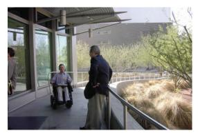
Suggestion: At the employees' exit just inside the building, the "push to open" button appears high. Repositioning the button and moving a table which was positioned there would make this exit more accessible.
