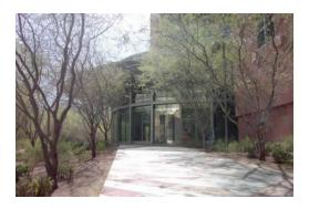
There was an automatic door opener button, but the position of the button required maneuvering around the door after pressing it because the door opened out (toward the individual). The timing of the automatic door opening and entry required more time than was available after pressing the button. Manual doors were somewhat heavy.
